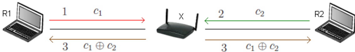
Figure 2.4: Transmission characteristics for COPE based network coding
