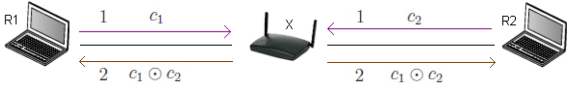
Figure 2.5: Transmission characteristics for Physical Layer Network Coding
