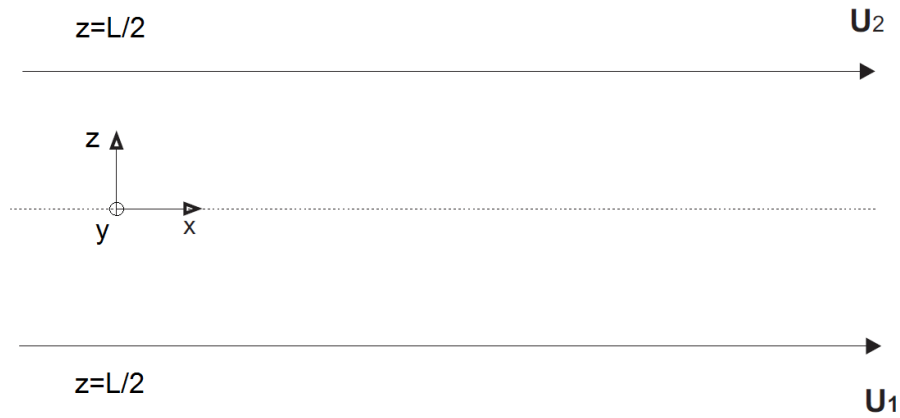
Figure 5.2: The cross section of channel geometry where the fluid is enclosed in the z -direction by two parallel plates with forcing only applied in the x -direction. The y -direction is perpendicular to this page and it is assumed that the fluid is periodic in this direction.
