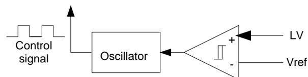
Figure 3.7 Block diagram of pulse-skip regulation
