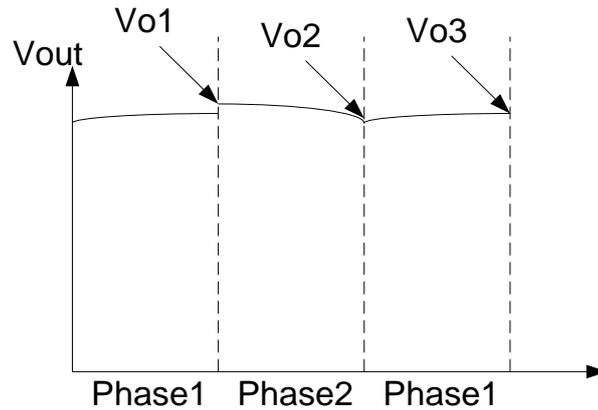
Figure 3.6 Timing diagram of DC-DC converter
