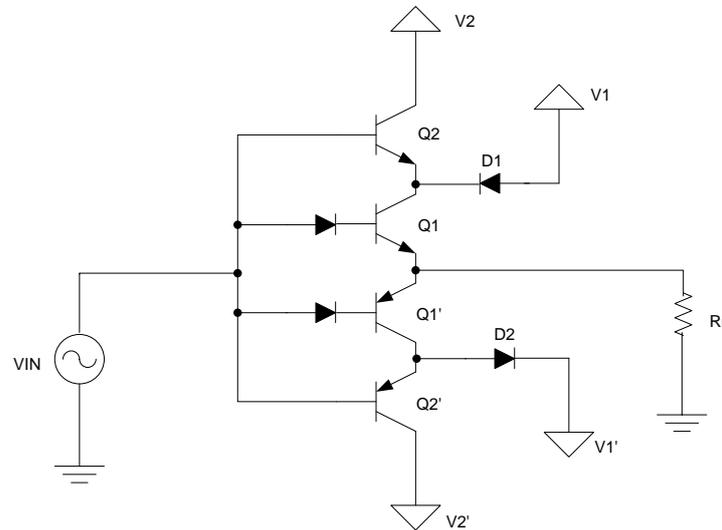
Figure 2.15 Basic configuration of Class G amplifier using diodes as control unit
