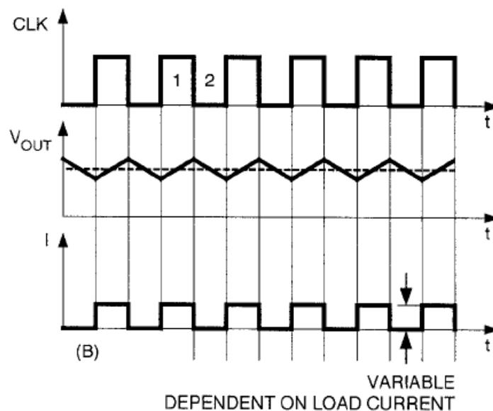
Figure 2.12 Constant-Frequency Regulation
