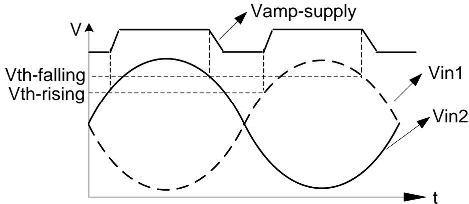
Figure 3.14 Transient response of Vin1, Vin2 and Vamp-supply
