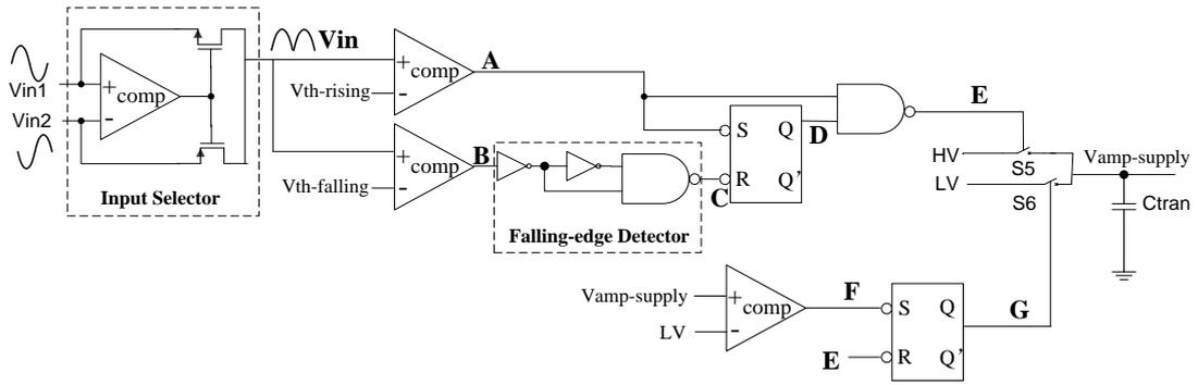
Figure 3.15 Block diagram of Supply Control Circuit
