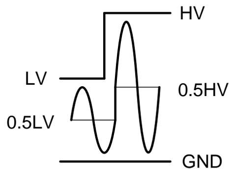
Figure 3.13 Waveform of output signal at different power supply rails
