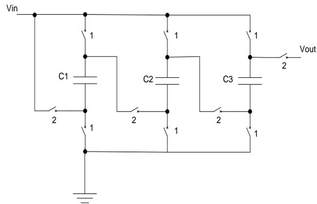
Figure 2.9 Basic structure of step-up switched-capacitor DC-DC converter (heap charge pump)
