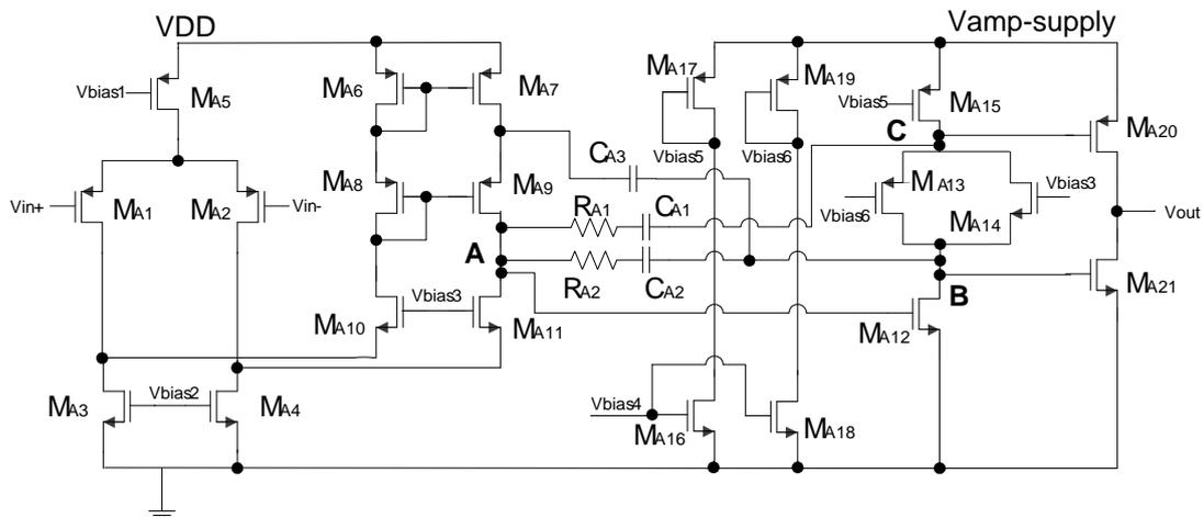
Figure 3.21 Schematic of the core amplifier
