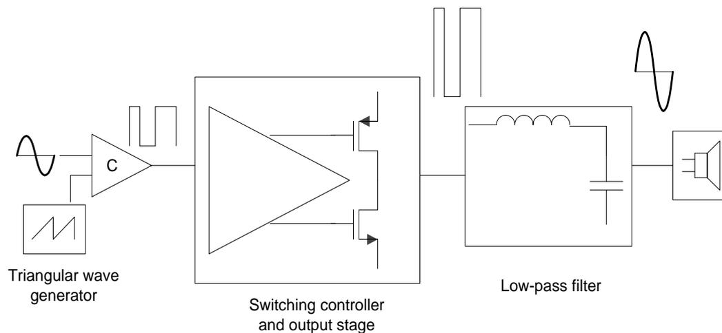
Figure 2.5 Basic configuration of a Class D amplifier
