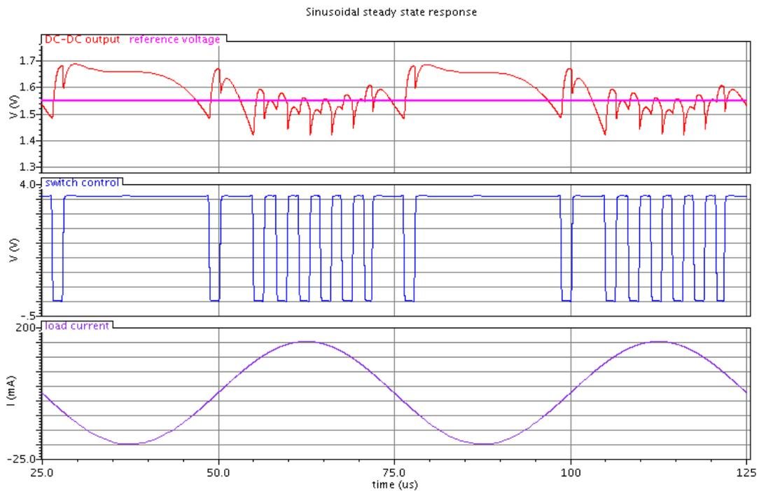
Figure 4.5 DC-DC regulated converter output and switch control signal
