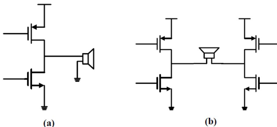
Figure 2.14 (a) Single amplifier (b) Bridge amplifier
