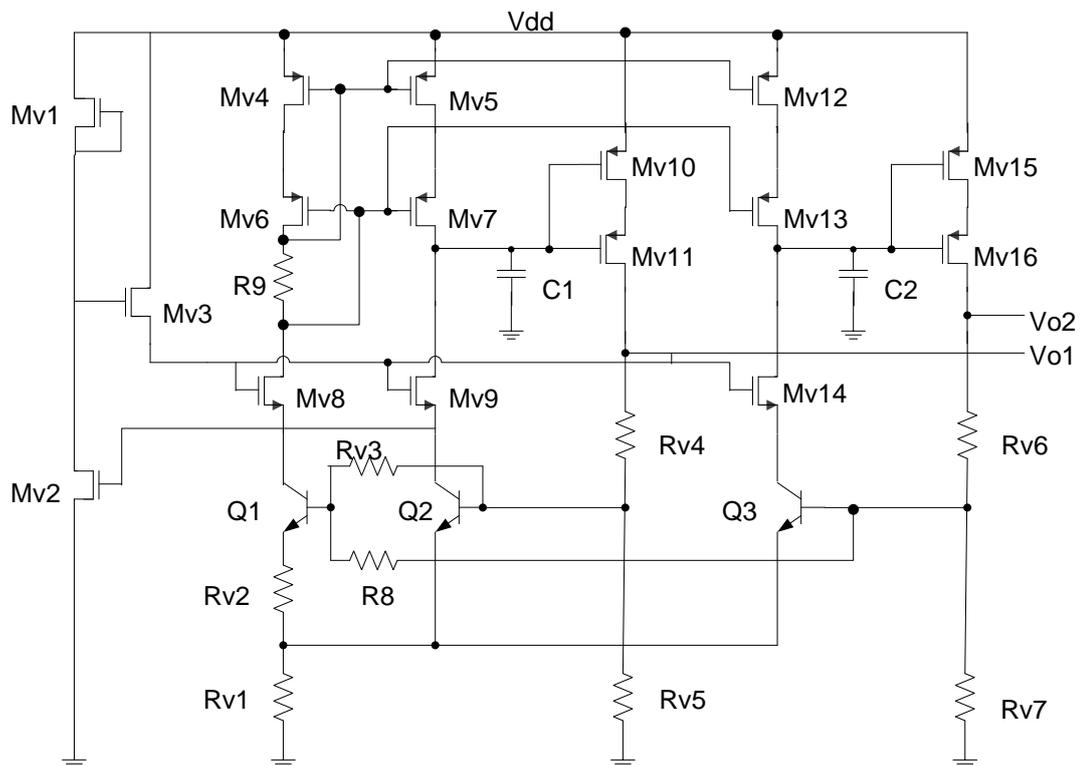
Figure 3.11 Schematic of the pseudo floating voltage generator
