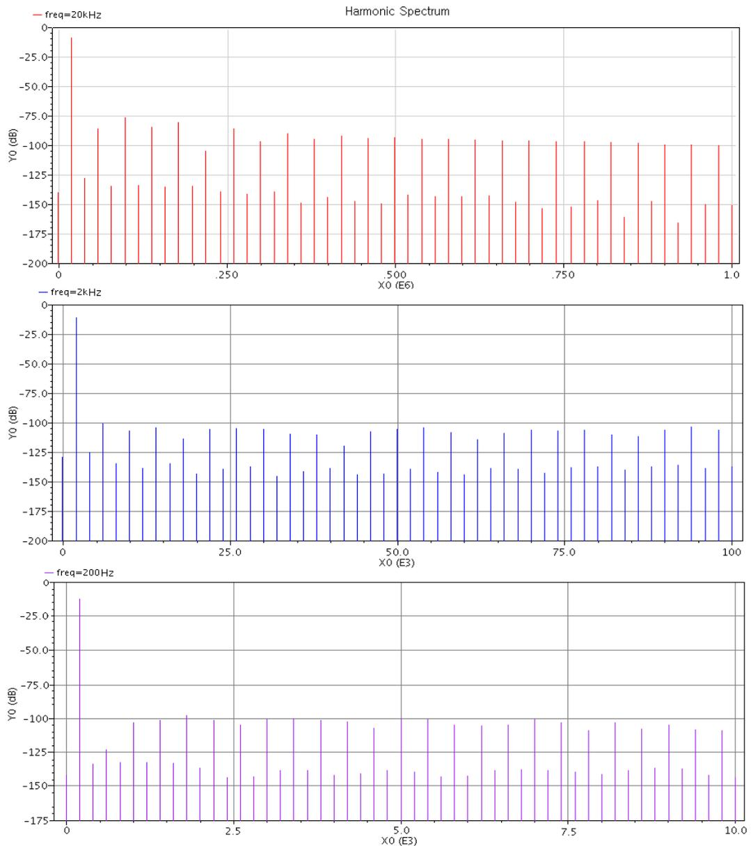
Figure 4.16 Harmonic Spectrum of frequency signal at 20kHz, 2kHz and 200Hz
