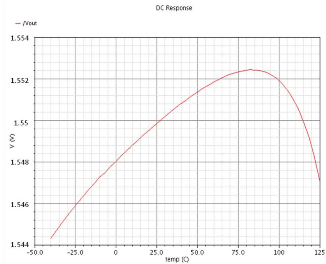
Figure 4.3 Voltage reference output voltage versus temperature
