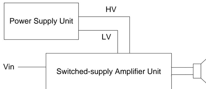
Figure 3.1 Simplified block diagram of Class G amplifier
