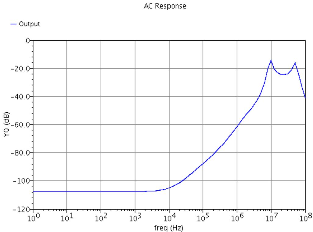
Figure 4.11 Simulated PSR of bridge amplifier
