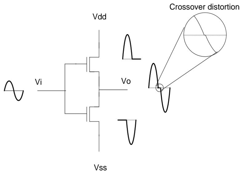
Figure 2.3 Basic configuration of Class B push-pull amplifier with crossover distortion
