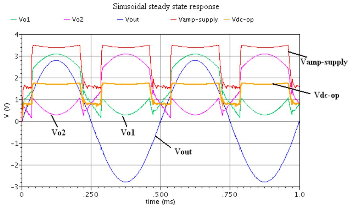
Figure 4.14 Sinusoidal steady state responses of large amplitude output voltage at high-voltage supply voltage
