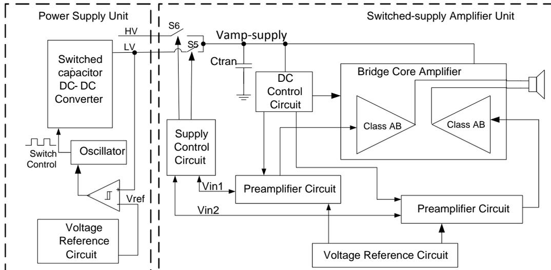
Figure 3.2 Overall block diagram of the proposed Class G amplifier
