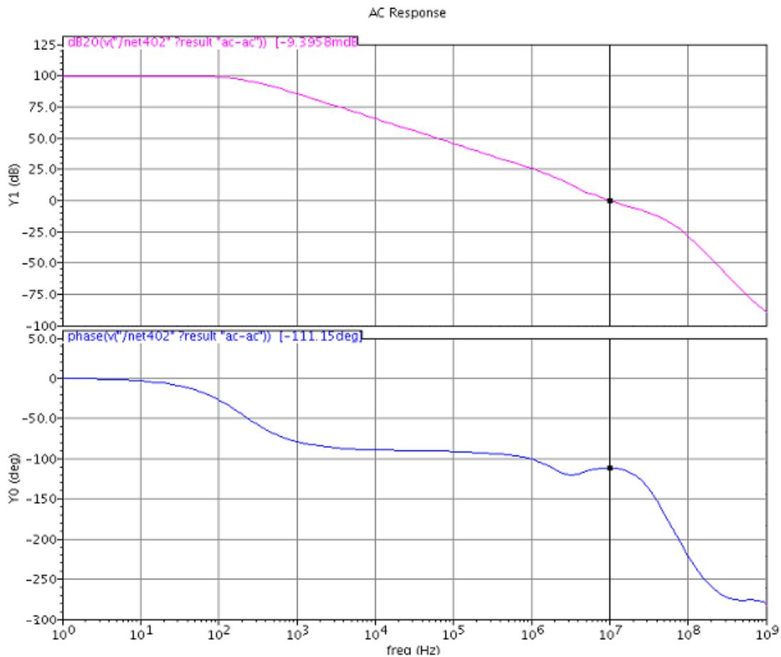
Figure 4.8 Frequency response of amplifier in low-voltage supply condition
