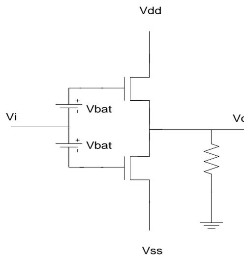
Figure 2.4 Basic configuration of a Class AB amplifier
