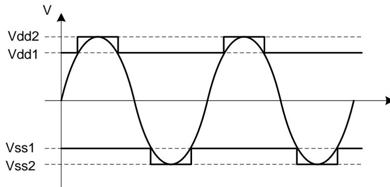
Figure 2.7 Waveform of Class G amplifier output
