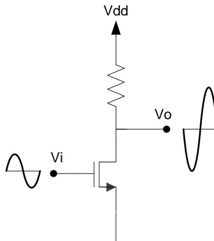
Figure 2.2 Basic configuration of a Class A amplifier
