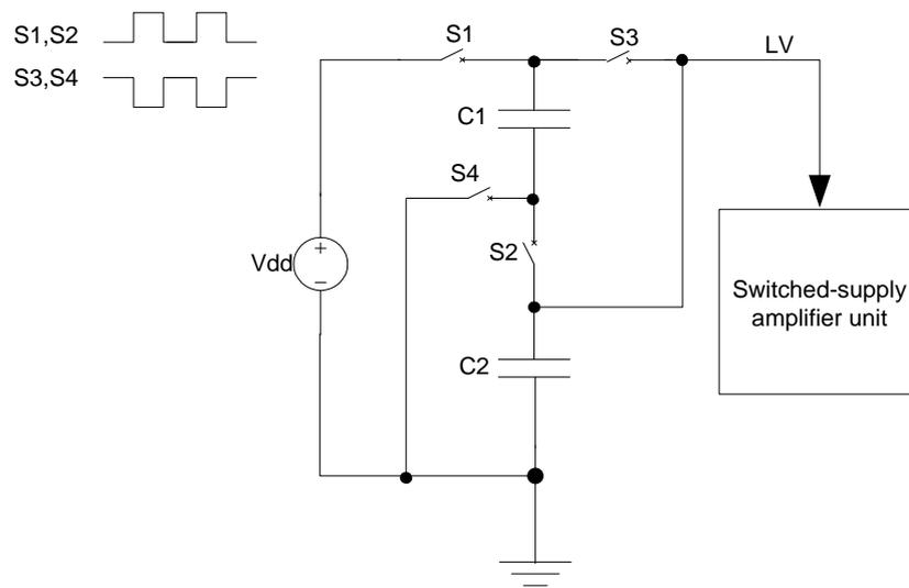
Figure 3.4 Configuration of the SC DC-to-DC step down converter
