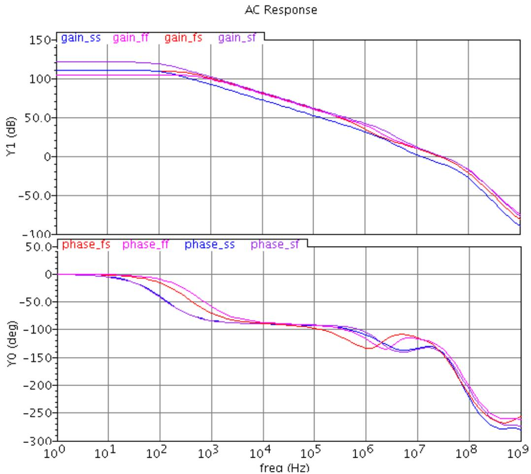
Figure 4.9 Frequency responses of amplifier at various process corners: ss (slow NMOS, slow PMOS), ff (fast NMOS, fast PMOS), fs (fast NMOS, slow PMOS) and sf (slow NMOS, fast PMOS)
