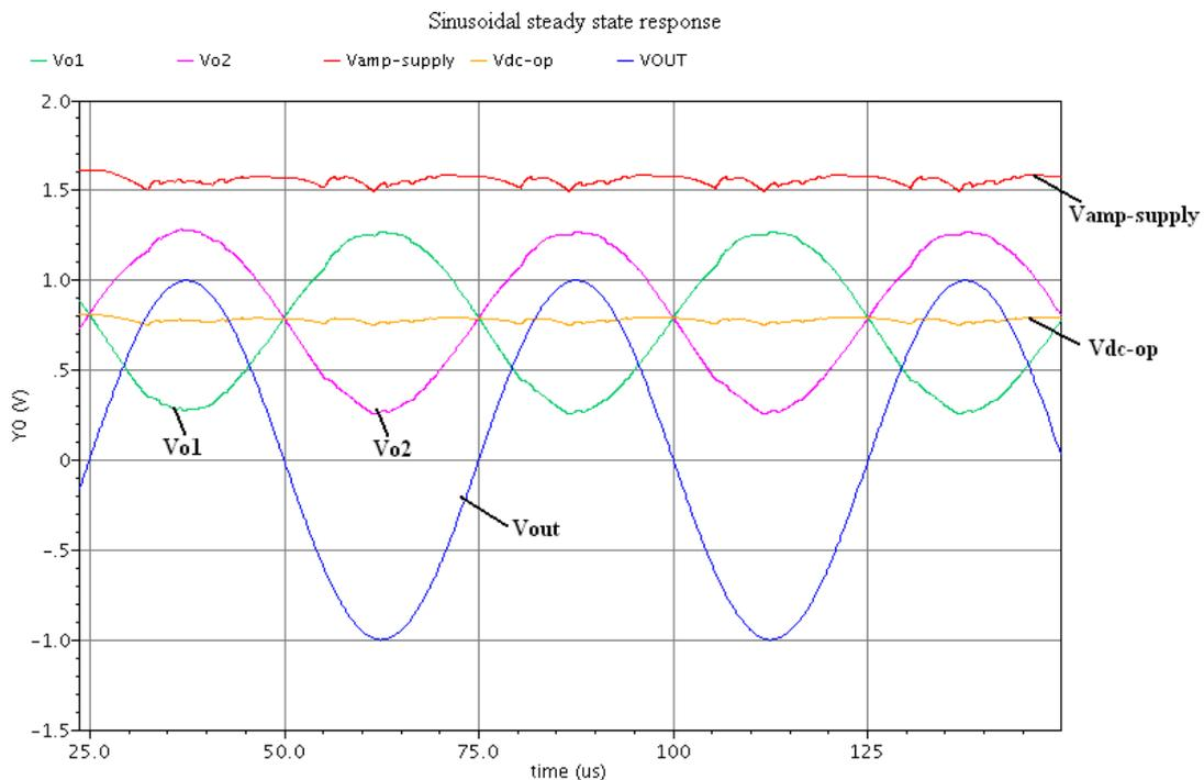
Figure 4.13 Sinusoidal steady state responses of small amplitude output voltage at low-voltage supply voltage
