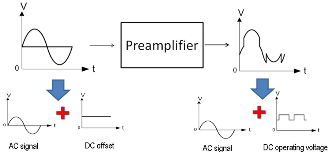
Figure 3.18 Pre-amplifier conceptual diagram
