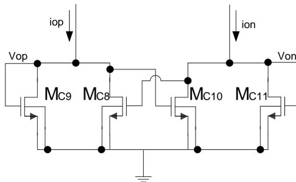
Figure B.1 Schematic of decision circuit in comparator
