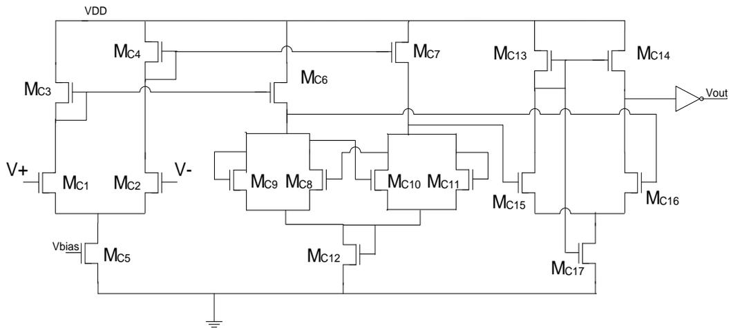
Figure 3.9 Schematic of the comparator
