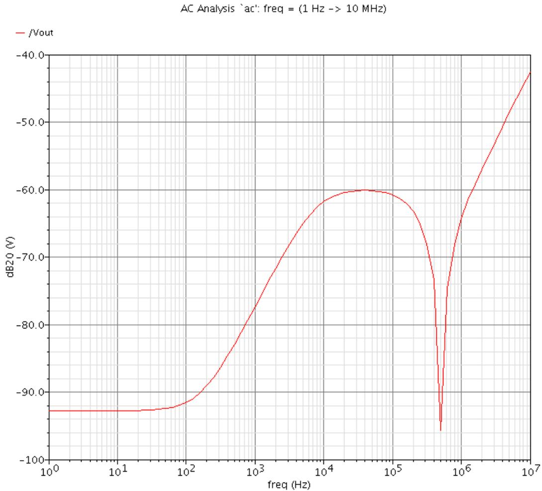
Figure 4.4 PSR of reference voltage
