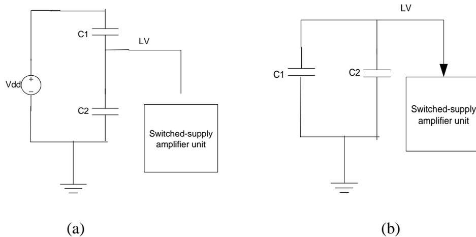
Figure 3.5 (a) Configuration of the DC-to-DC converter at phase 1
