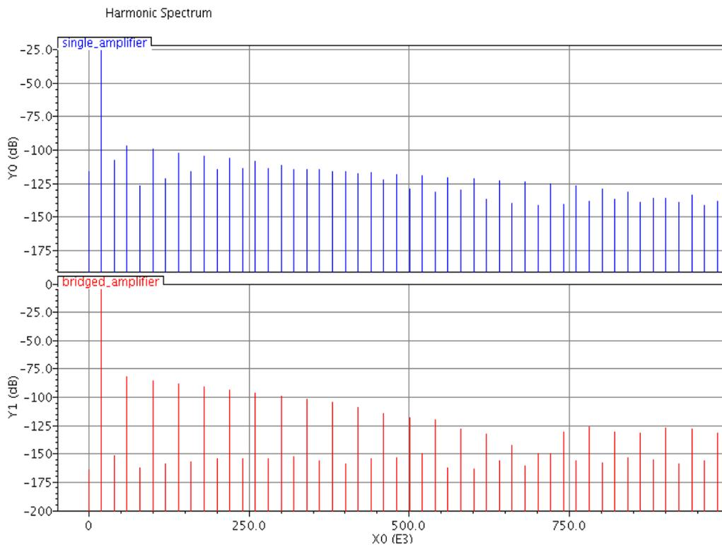
Figure 4.12 Harmonic spectrum of single amplifier and bridge amplifier
