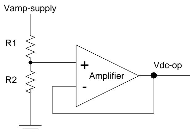
Figure 3.17 Configuration of the DC control circuit
