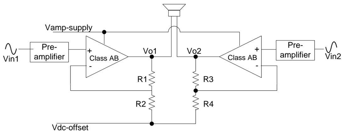
Figure 3.20 Basic configuration of the bridge amplifier
