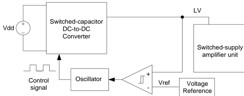
Figure 4.1 Block diagram of the power converter system
