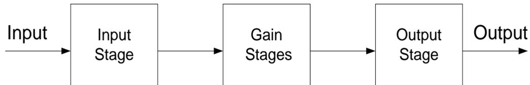
Figure 2.1 Structure of the linear amplifier
