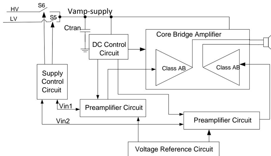
Figure 3.12 Block diagram of the switched-supply amplifier unit
