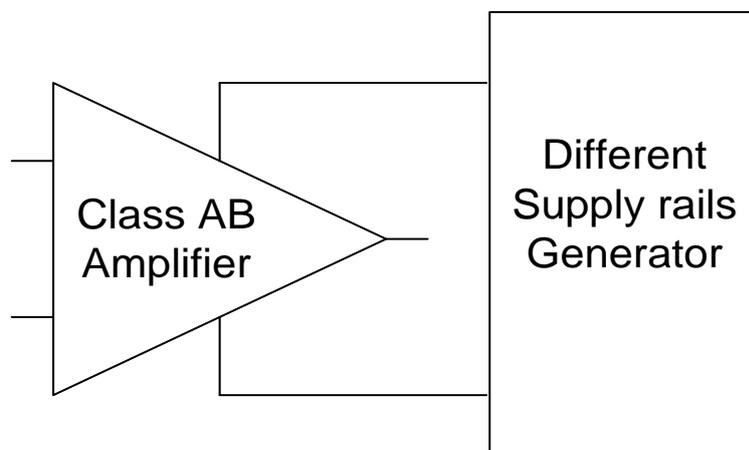
Figure 1.1 Block diagram of a typical Class G power amplifier
