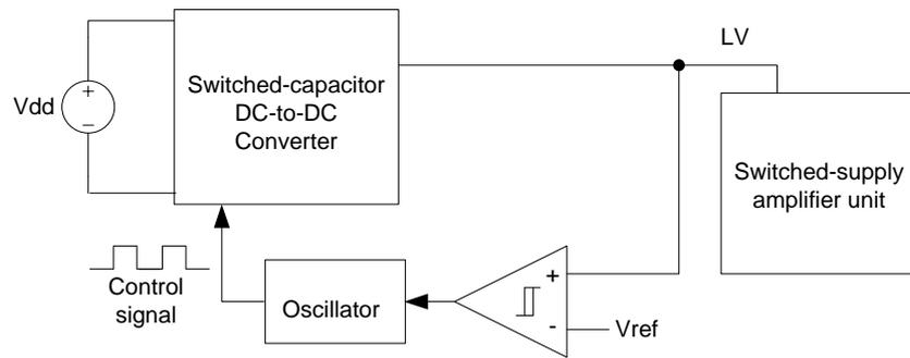
Figure 3.3 Block diagram of the power converter system
