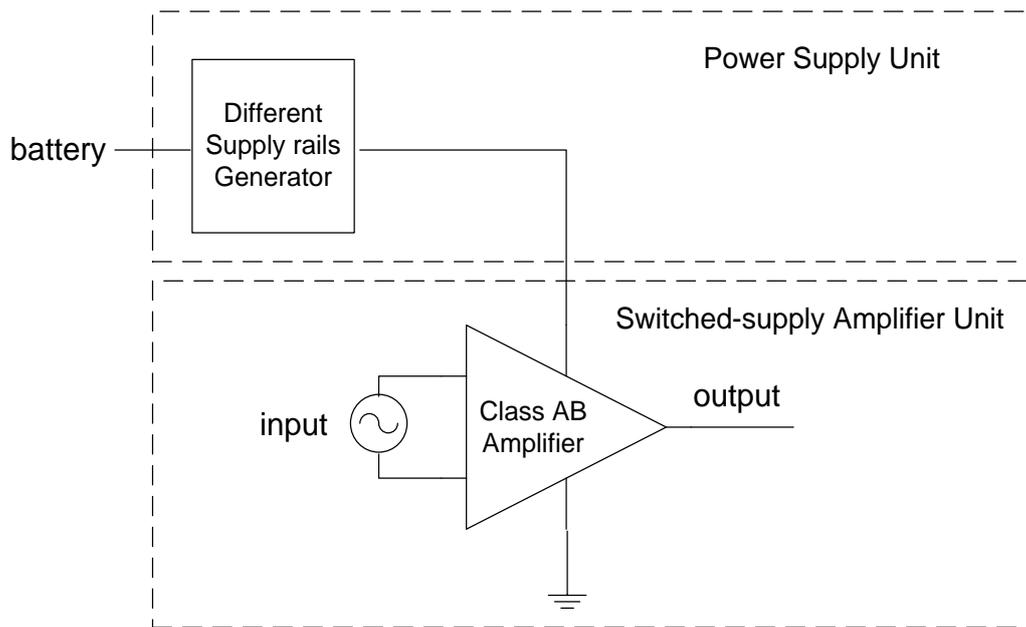
Figure 2.8 Architecture of Class G power amplifier
