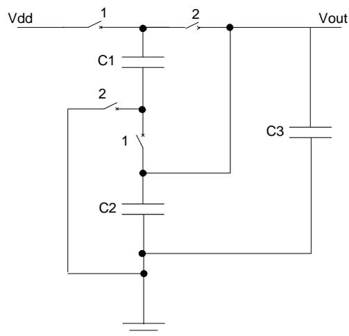
Figure 2.10 Basic structure of step-down switched-capacitor DC-DC converter.
