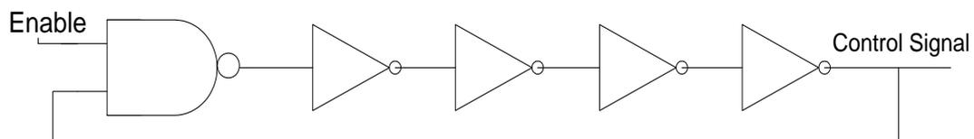
Figure 3.8 Schematic of the ring oscillator
