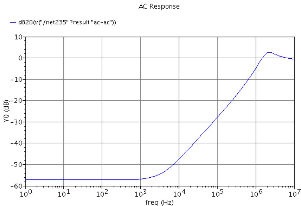
Figure 4.10 Simulated PSR in low-voltage supply condition
