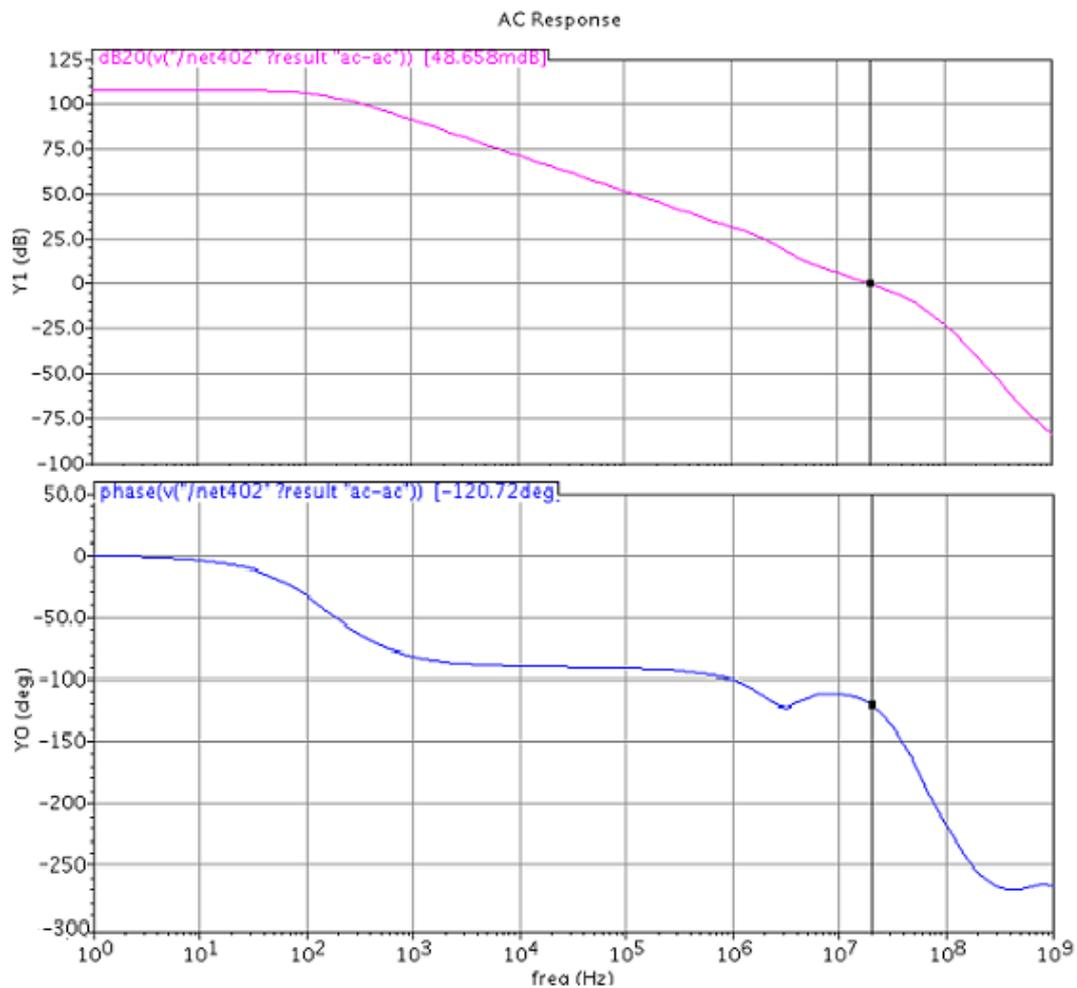
Figure 4.6 Frequency response of amplifier in high-voltage supply condition
