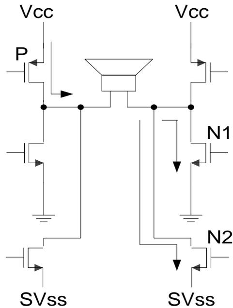
Figure 2.16 Basic configuration of Class G amplifier without diodes
