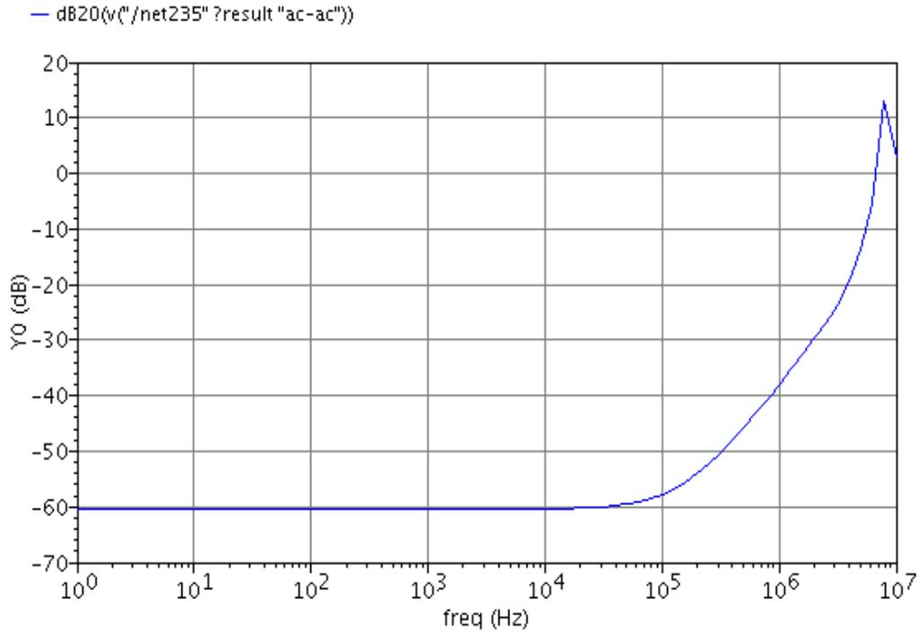
Figure 4.7 Simulated PSR in high-voltage supply condition
