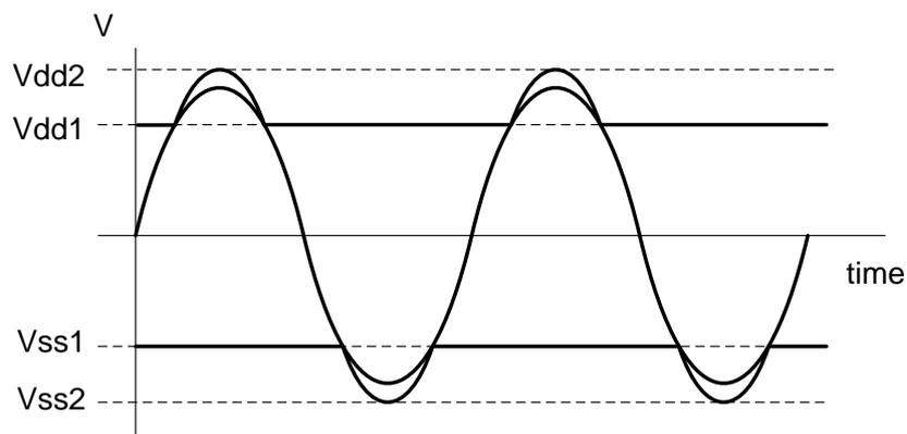
Figure 2.6 Waveform of Class H amplifier output
