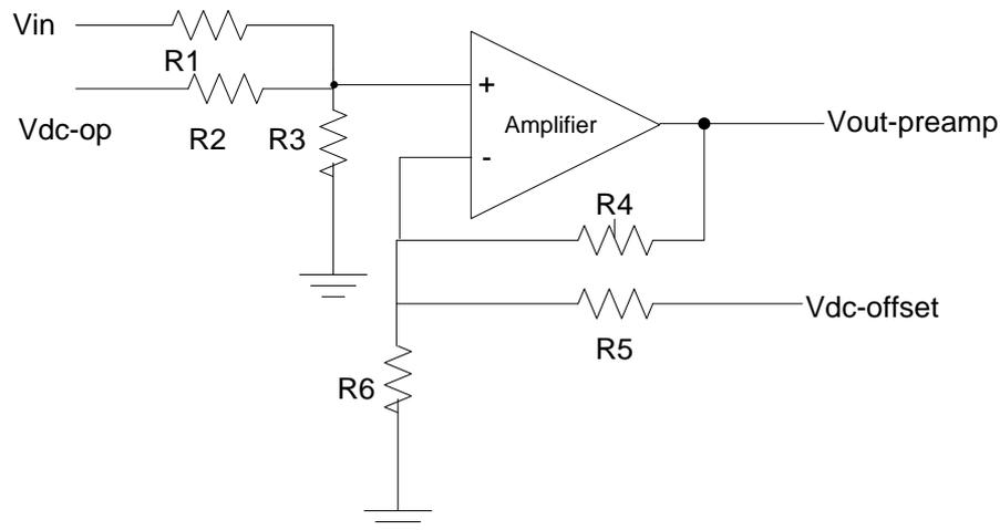
Figure 3.19 Configuration of preamplifier
