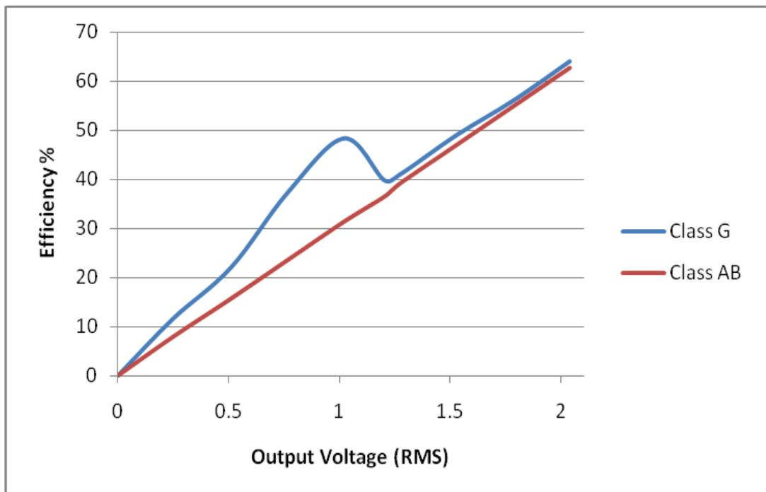
Figure 4.17 Power efficiencies of Class G amplifier and Class AB amplifier versus output voltage
