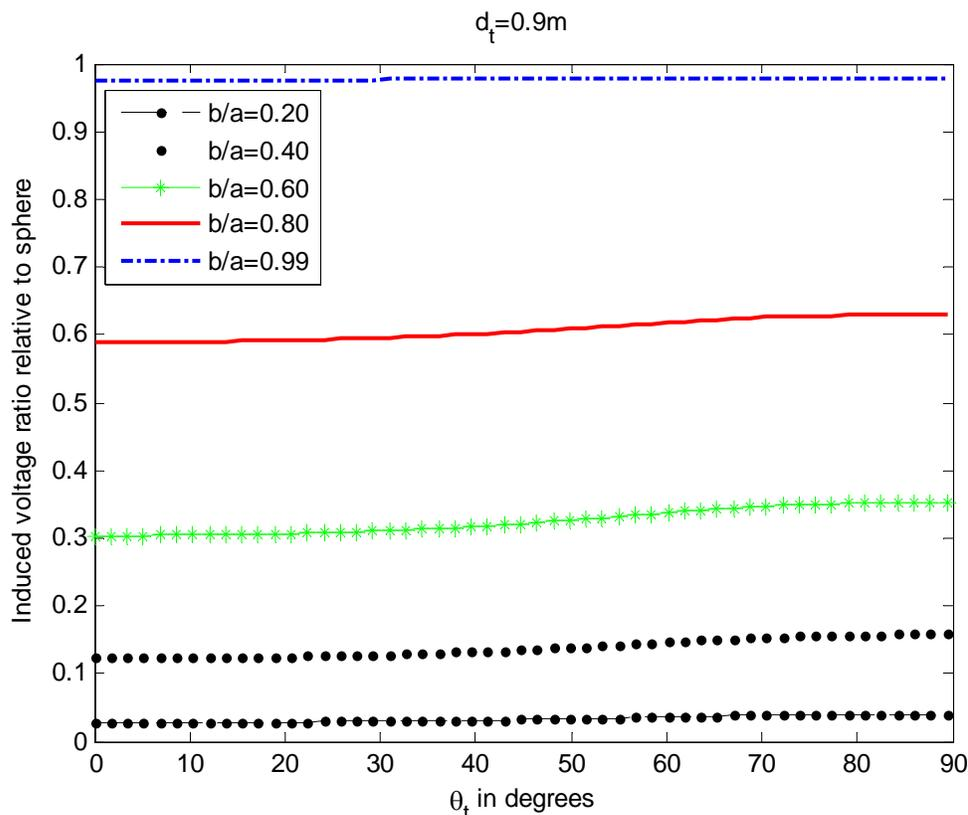
Figure 5-5: Angular scan of the total induced voltage for a conducting spheroid buried vertically relative to its corresponding sphere with different axes aspect ratio for the depth  $d_t=0.9m$
