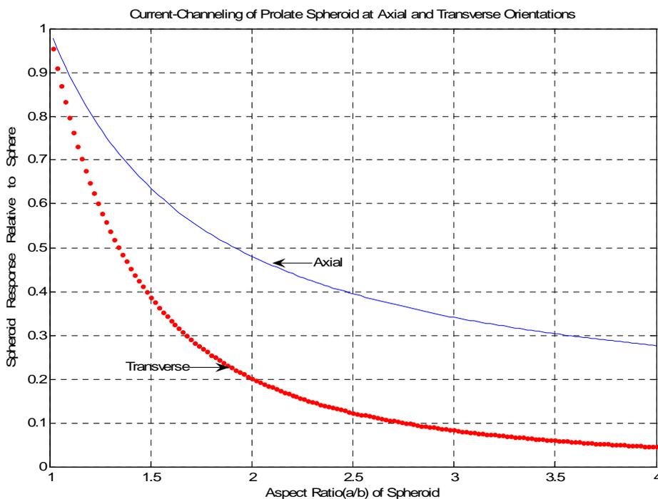
Figure 4-3: Current-Channelling polarizabilites of Prolate at two orientations
