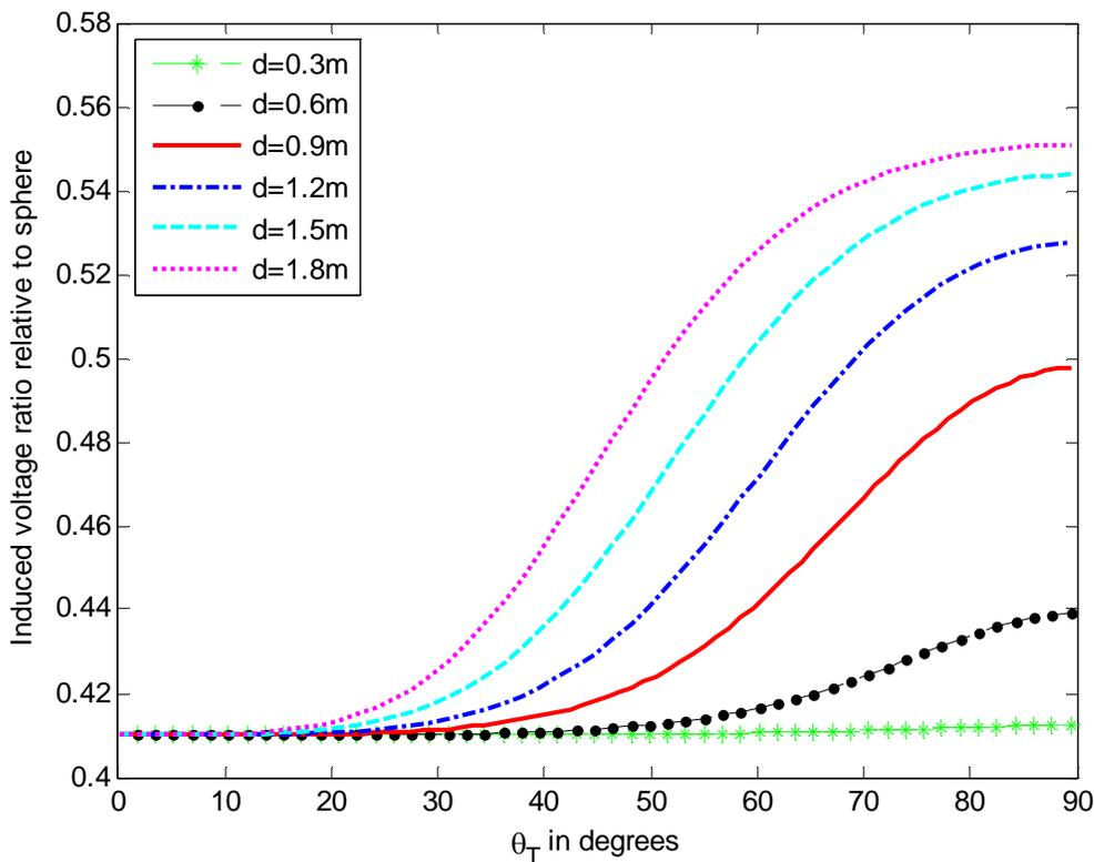
Figure 5-4: Angular scan of the total induced voltage for a conducting spheroid relative to its corresponding sphere with the axes aspect ratio of 0.6 at different depths for the configuration depicted in Figure 4.6
