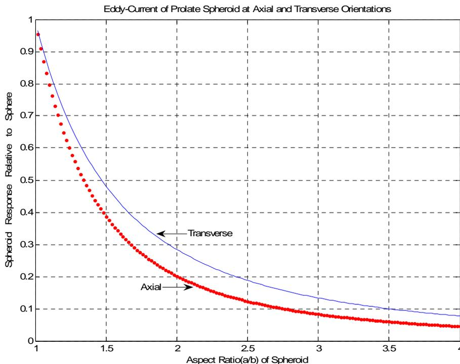
Figure 4-2: Eddy-current polarizabilities of Prolate at two orientations
