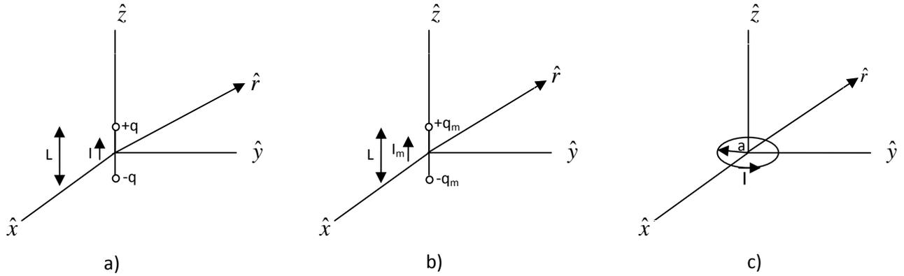
Figure 2-2: a) Small electric current element or electric dipole. b) Short magnetic current element or magnetic dipole. c) Small loop of electric current.
