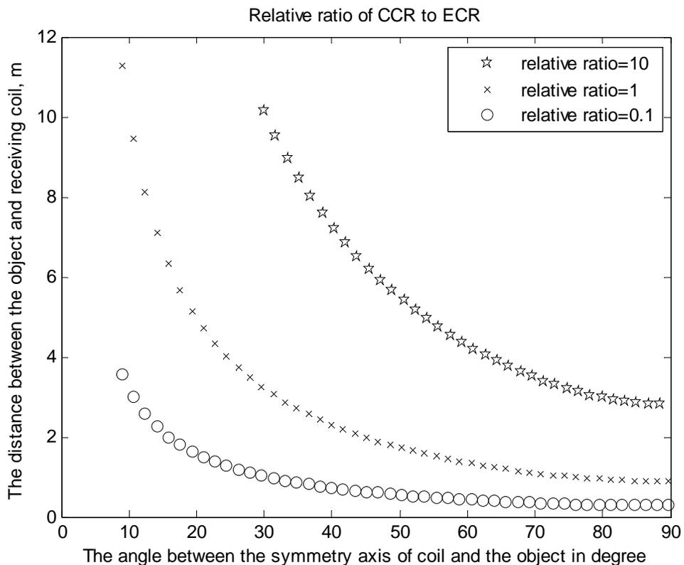
Figure 3-3: Relative ratio of CCR to ECR at different depths for a spherical conducting object
