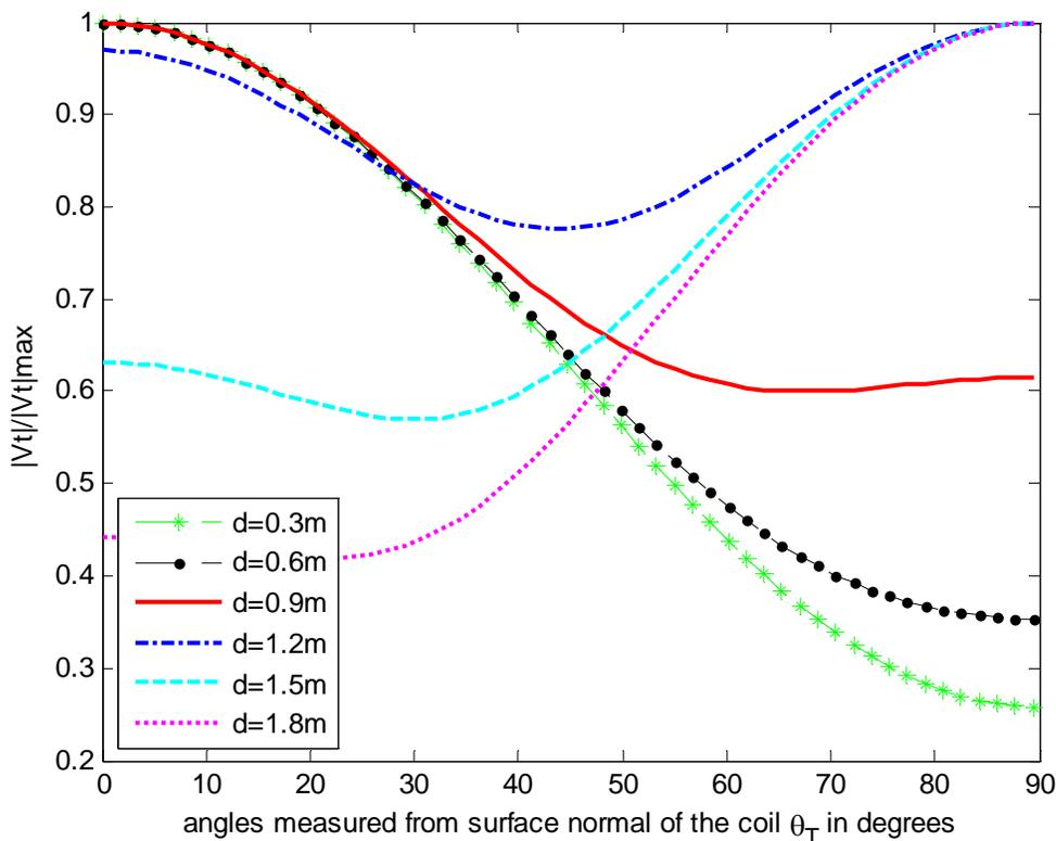
Figure 5-1: Angular scan of normalized induced voltage for a spherical conducting marine mine at different depths
