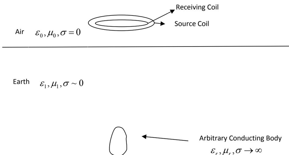
Figure 2-1: Configuration of general EMI system with a buried conducting object
