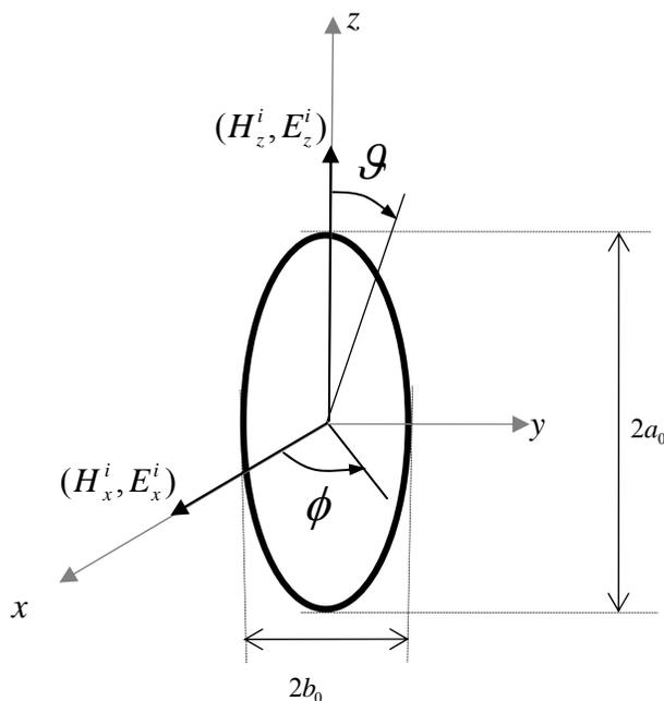
Figure 4-1: A perfectly conducting prolate spheroidal object being excited with incident electric and magnetic fields
