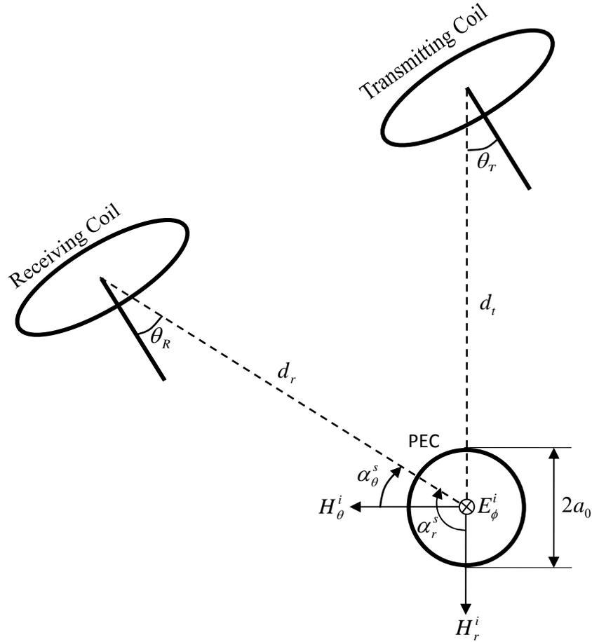
Figure 3-2: General configuration of mine detection through separate transmitting and receiving coils
