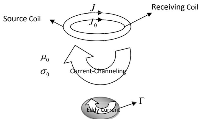
Figure 2-3: Illustration of Eddy-Current and Current-Channelling response in a conducting background environment
