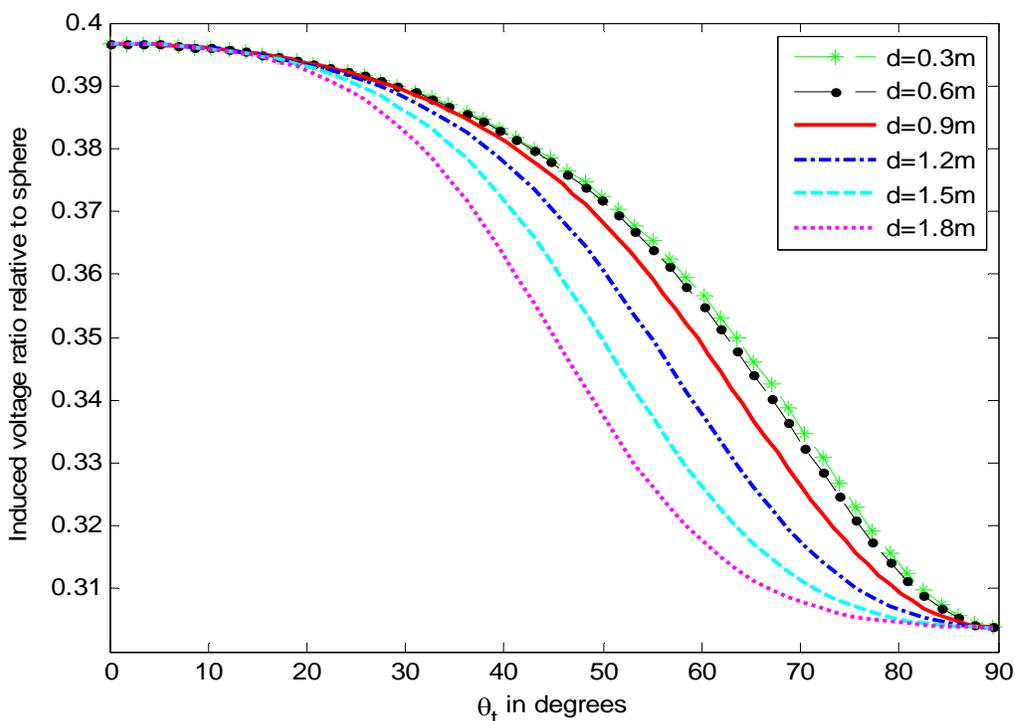
Figure 5-3: Angular scan of the total induced voltage for a conducting spheroid relative to its corresponding sphere with the axes aspect ratio of 0.6 at different depths for the configuration depicted in Figure 4.5
