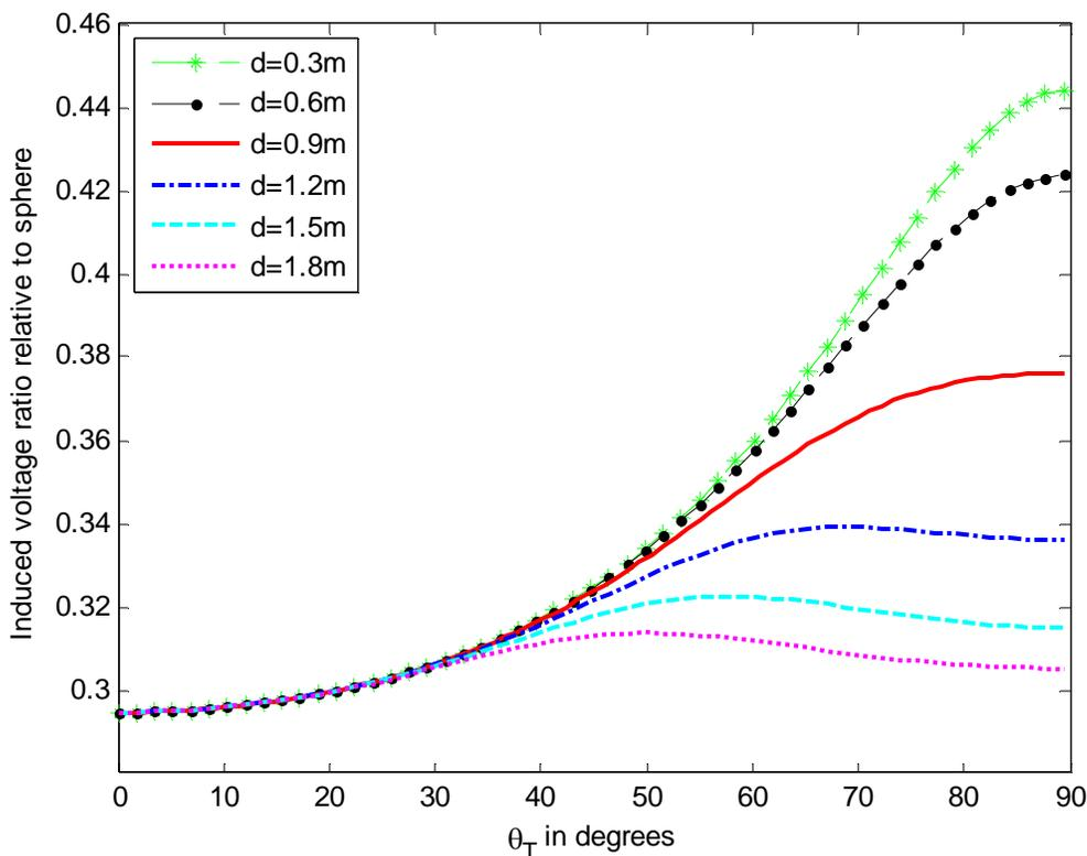
Figure 5-2: Angular scan of the total induced voltage for a conducting spheroid relative to its corresponding sphere with the axes aspect ratio of 0.6 at different depths for the configuration depicted in Figure 4.4
