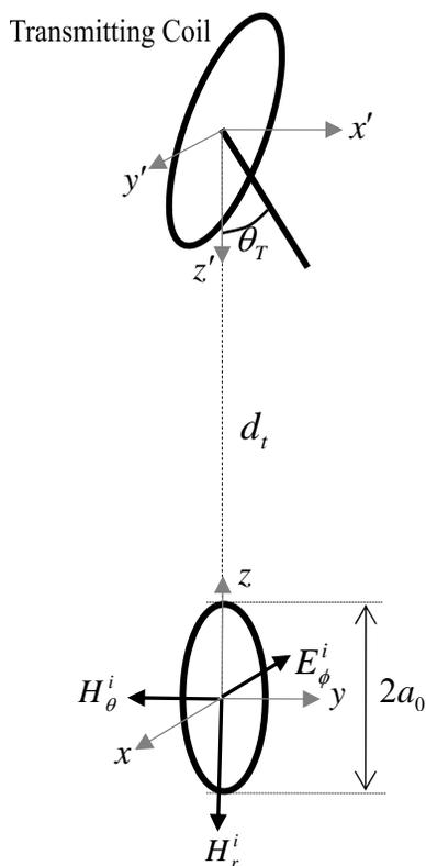
Figure 4-4: The first representative modes of a spheroidal mine embedded in the conducting medium
